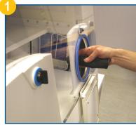
Roll a replacement membrane and insert into the workstation through the membrane that is not being replaced.
