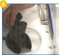
Carefully peel the existing membrane out of the retaining slot in the membrane carrier.
