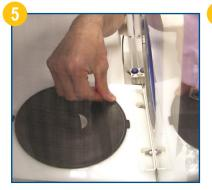
Position the replacement membrane into the retaining slot, carefully pressing the membrane into place along it's entire edge. Take special care that the location tab engages with the small pocket at the lower edge of the carrier.
